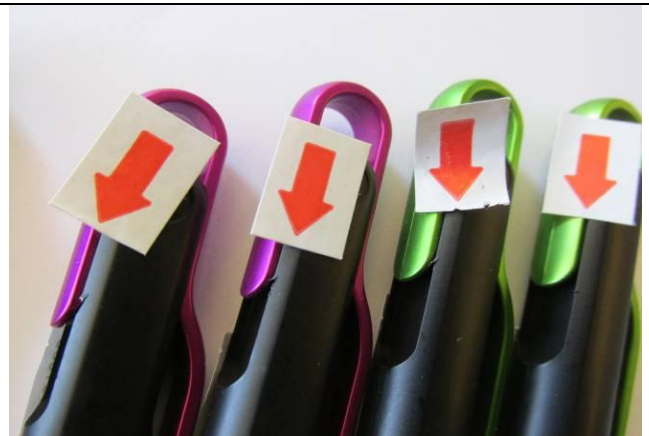
DEFECT-CUTTING MARK (MINOR)
