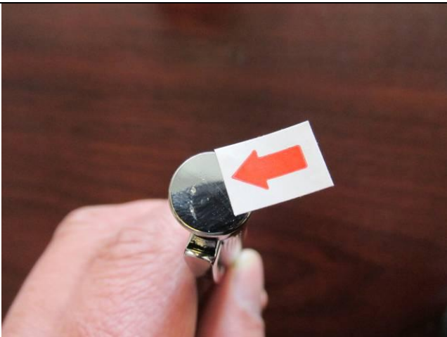
DEFECT---DENT MARK ON UNIT (MINOR)
