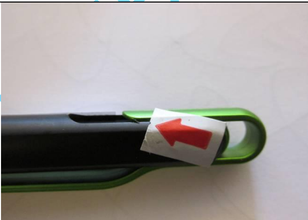
DEFECT-CUTTING MARK (MINOR)
