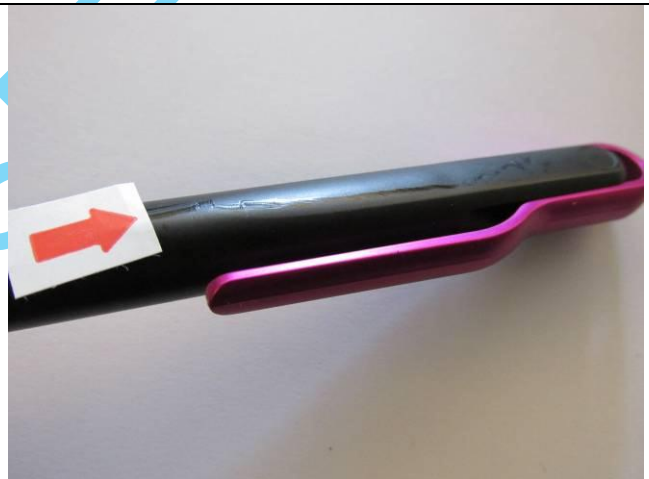
DEFECT---SCRATCH MARK ON UNIT (MINOR)
